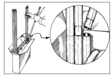
3. Lift top section of screen from carton and connect 3 tubes on left and then connect 3 tubes on right.
